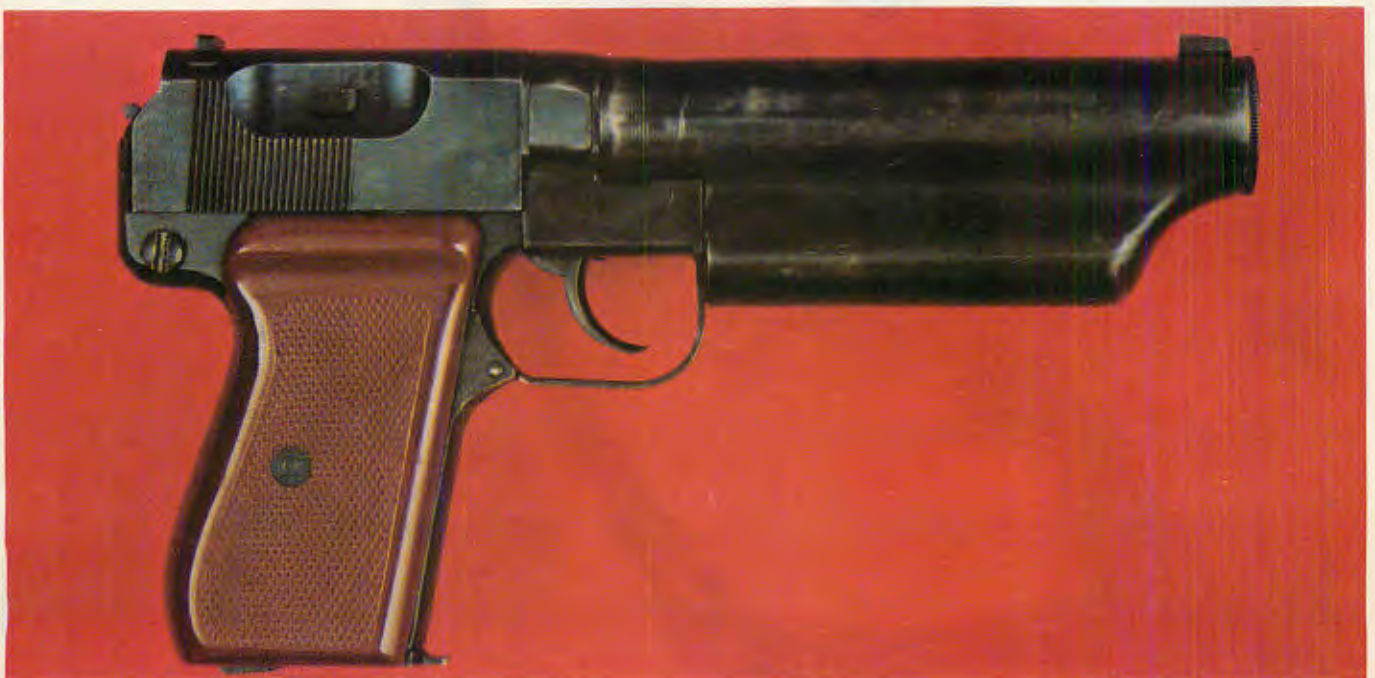
Clean lines give model 64 a modern look but accentuate flimsy appearance of trigger guard. Hanging trigger looks inappropriate. Note magazine release on bottom.
